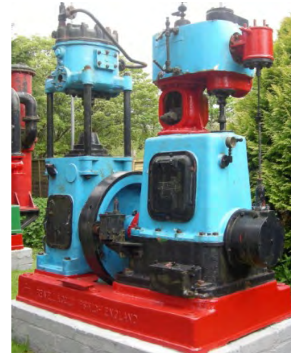
Reader steam engine connected to Reavell pump, on static display at Poldark Mine Museum (Courtesy gracesguide.co.uk).
